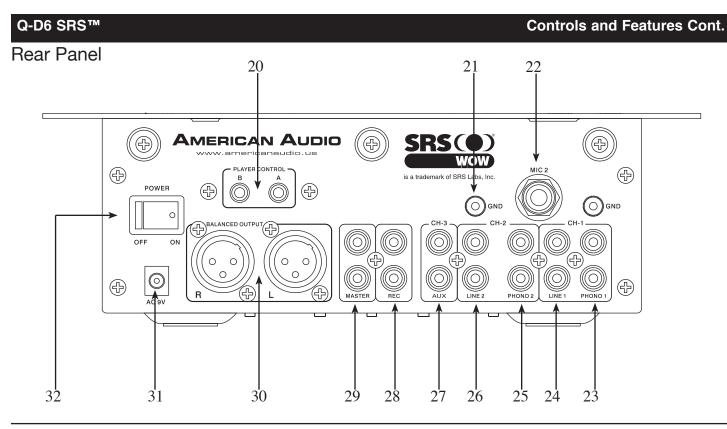
**20. PLAYER CONTROL** - These jacks are used to control the "Q-Start" function between the mixer and a compatible American Audio CD Player. Input mini plugs from CD player controller into these jacks, input CD 1 into jack A and CD 2 into jack B.
